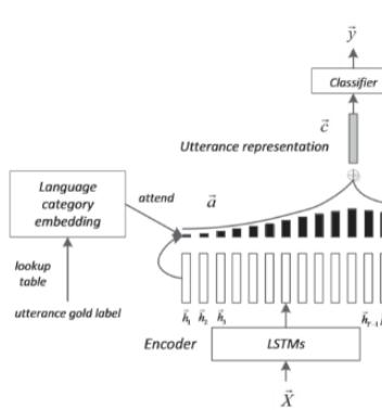
Figure 1: The Architecture of attention-based recurrent neural network.
