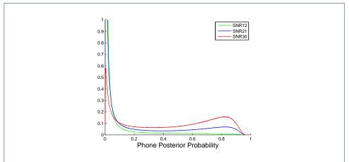
Figure 3 Distribution of the values  $P(v|x_t)$  on the development set, with white noise mixed at different SNRs.
