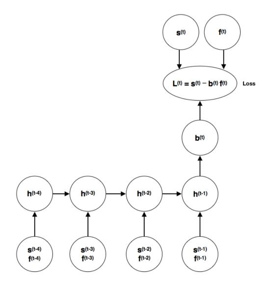
Note that inputs are past returns of spot and futures,  $b^{(t)}$  is the predicted best hedge ratio. The loss is equivalent to the random return to this portfolio  $x^{(t)} = s^{(t)} - b^{(t)}f^{(t)}$ , since we want to make  $x^{(t)}$  as small as possible. The Model was implemented with Tensorflow in Python.
