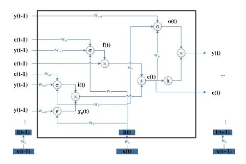
Figure 2: The architecture of an LSTM cell used in the LSTM-DSSM
