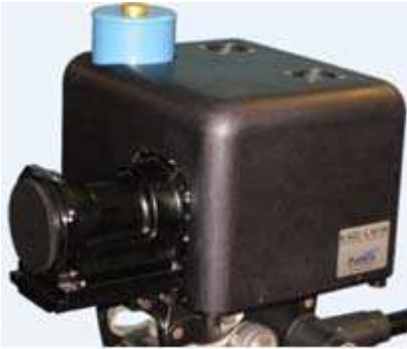
Figure 2: Polarimetric LWIR imager used in this study.
