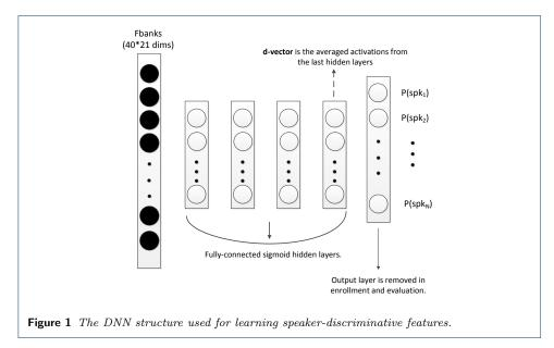
Figure 1 presents the DNN structure used for the speaker-discriminative feature learning. Following the convention of ASR, the input layer involves a window of 40-dimensional Fbanks. In this work, the window size is set to 21, which was found
